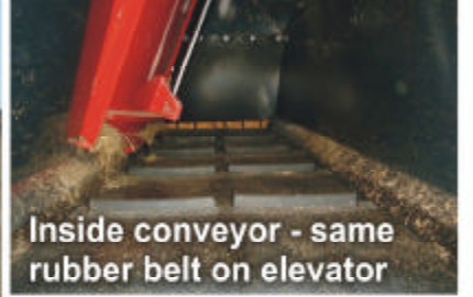
Inside conveyor - same rubber belt on elevator
